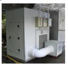
The controlled-environment facilities can adjust the temperature, humidity and carbon dioxide concentration.
