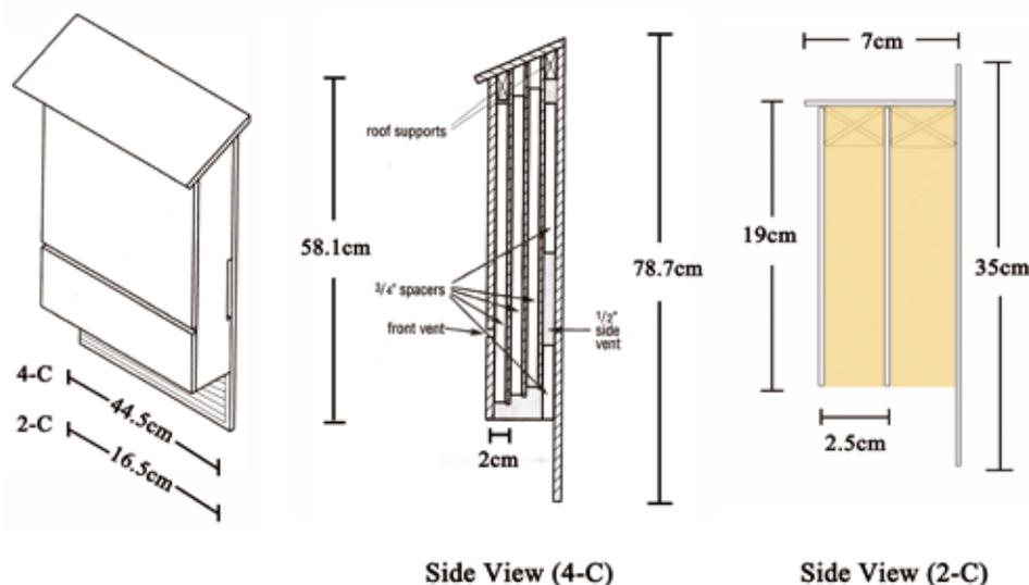
Fig 30. Designs & dimensions of the 2-chambered (2-C) and the 4-chambered (4-C) bat-boxes. (Reprinted with permission from Tuttle *et al.* (2005), Bat Conservation International, for the 4-chambered bat-box.)
