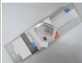
42. Soil EC tester For rapid determination of soil electrical conductivity (EC).
