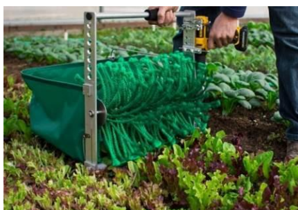
15. Handheld harvester For harvesting crops.
