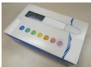
43. Nitrate ion meter For rapid determination of nitrate ion concentration in samples.
