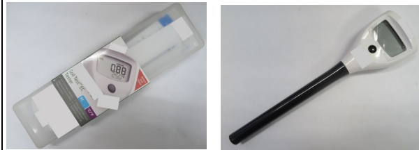
42. Soil EC tester For rapid determination of soil electrical conductivity (EC).
