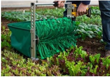
15. Handheld harvester For harvesting crops.
