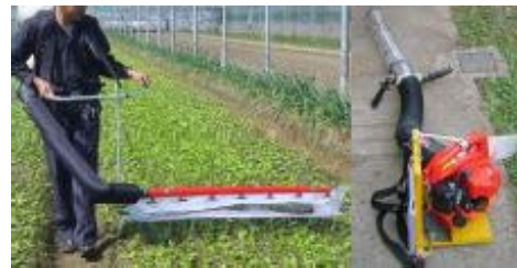
28. Insect Suction Trap Catcher For trapping tiny pests.
