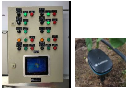
48. Remote monitoring and control systems for farms For remote monitoring of the farm environment and control of various equipment.
