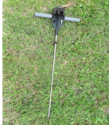
46. Soil compaction tester For measurement of soil compaction level
