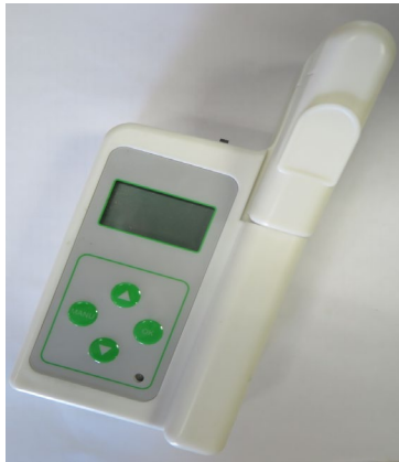
47. Chlorophyll meter For non-invasive measurement of chlorophyll content, leaf surface temperature and moisture content of plants.
