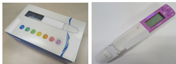
44. Potassium ion meter For rapid determination of potassium ion concentration in samples.
