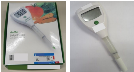
41. Soil pH tester For rapid determination of soil pH values.
