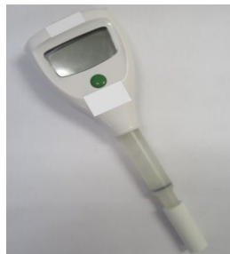
41. Soil pH tester For rapid determination of soil pH values.
