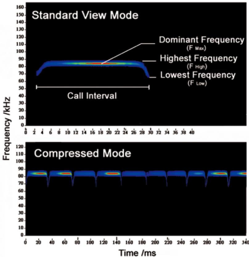
Fig 26. Sonogram (in compressed mode and standard view) of the Chinese Horseshoe Bat by Pettersson D240X bat detectors and Sonobat v.2.6.2.  $F_{max}$  is dominant frequency with highest energy distributed from a power spectrum (red color);  $F_{high}$  is highest frequency of the extracted call;  $F_{low}$  is the lowest frequency of the extracted call; INT is the call interval between extracted calls.
