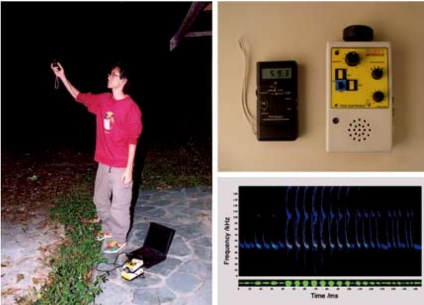
Fig 24. Bat acoustic monitoring by using bat detectors. a) Pettersson D240X and Anabat II bat detectors; b) Sonogram by Sonobat v.2.6.2.
