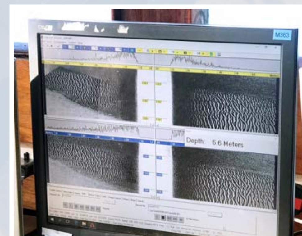
▲ Side Scan Sonar image showing sand ripples on seabed
