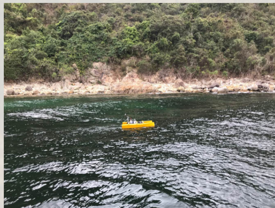
▲ Conducting shallow water survey by water drone
