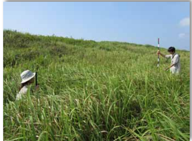
Fig. 3. An observer (left), through the sighting pole, is taking a visual obstruction measurement with a Robel Pole (right).
