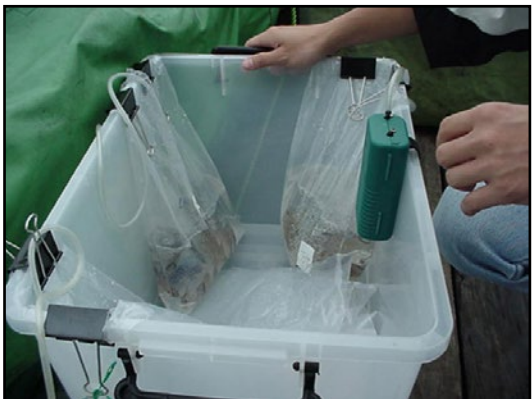
Figure 81. Battery operated aerators to keep fish samples alive en-route to the laboratory.
